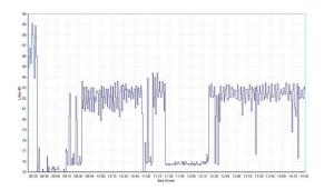
To the left is a noise graph downloaded from a noise dosimeter. It shows the noise levels that the worker was exposed to over the course of the day. Such graphs can be useful to identify which parts of the day are the noisiest.
